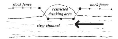
Vulnerable banks can be fenced. The riverbank fence is built into the river at one point, but not into the main channel, a good place is on the inside of a bend.
