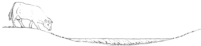
over-widened, shallow, muddy channel
